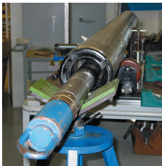
DSS/RMM alignment testing in a shore-based laboratory.
