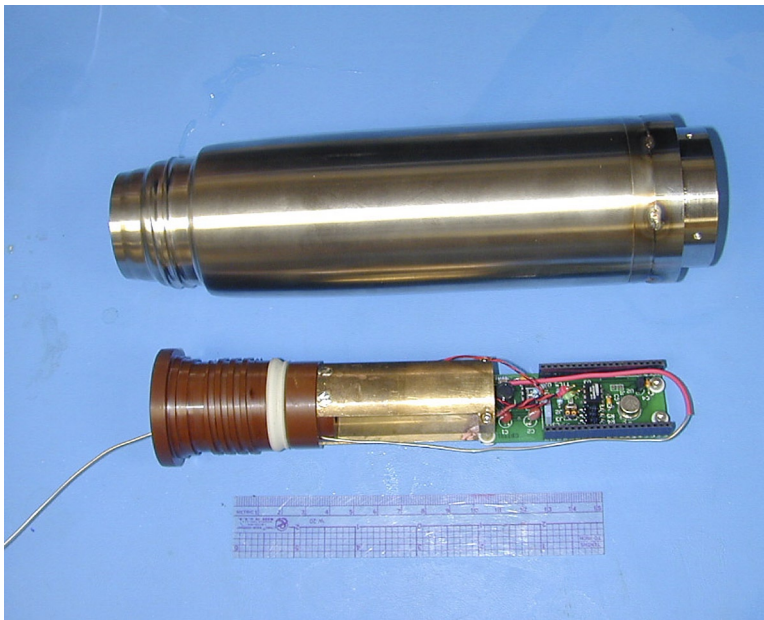
Figure 1. CB-TT electronics and dewar. Note that the datalogger board is removed in this photo.
