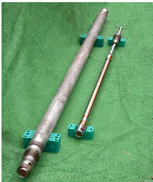
During assembly, the electronic components of the HTT (right) are placed inside the pressure case.
