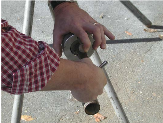
Figure 11. Rotating the "T" handle with the spring loaded plunger pushed in.
