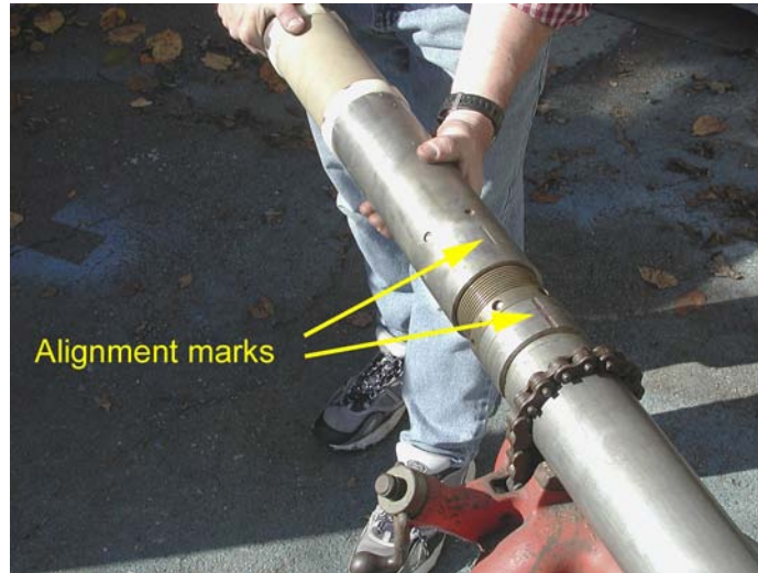
Figure 20. Alignment of the CB-RMM battery section and antenna mandrel.
