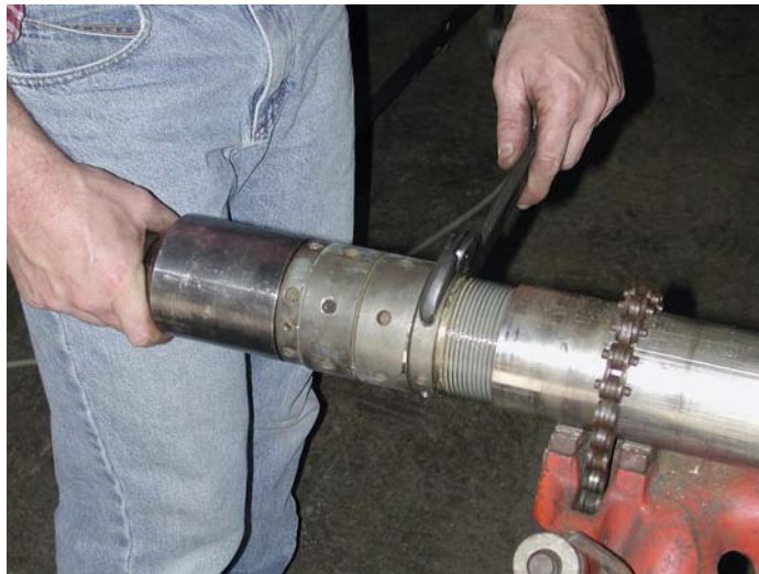
Figure 3. Loosening the bottom of the DSA-XM.
