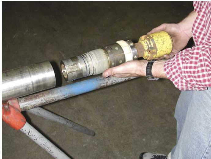
Figure 4. Removing the upper end of the DSA-XM.
