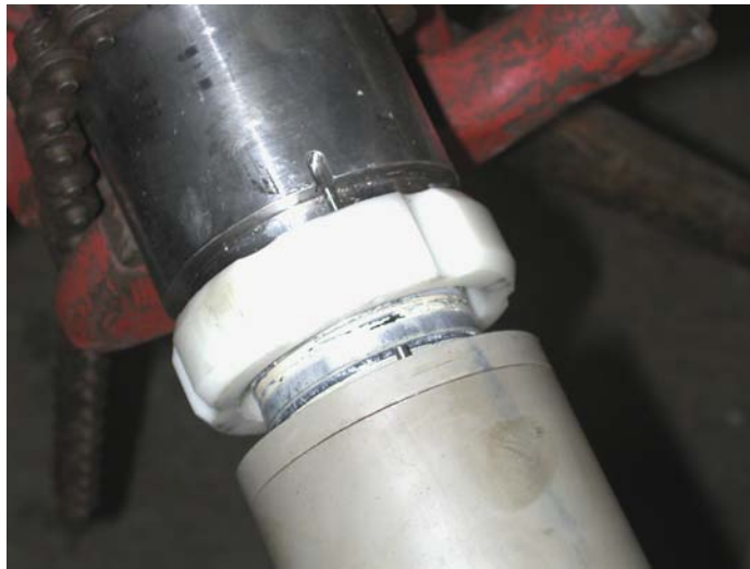
Figure 15. Separation of the antenna coil assembly from the mandrel.
