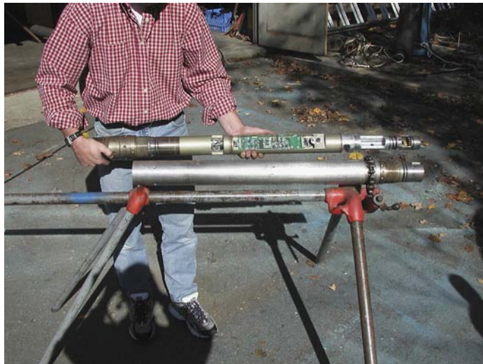
Figure 2. The CB-RMM. Note the Schlumberger-type connection on the section of the tool in the foreground.
