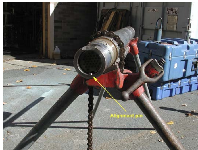
Figure 10. The top of the CB-RMM housing; the yellow arrow shows the location of the alignment pin.
