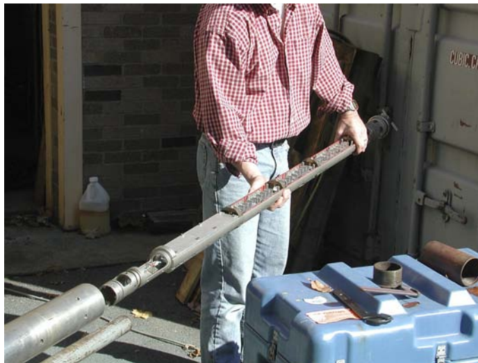
Figure 12. Pulling the chassis of the CB-RMM out of the lower end of the tool.
