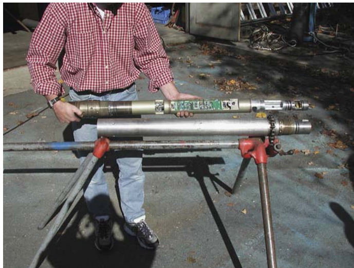
Figure 7. Housing and chassis of the CB-RMM.
