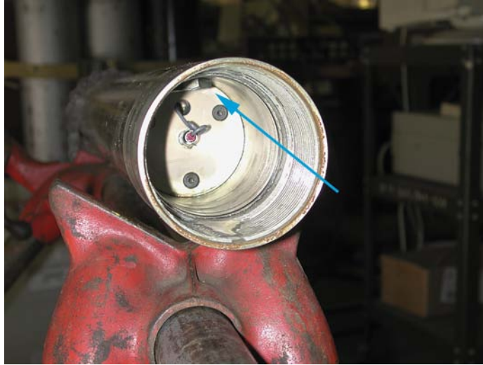
Figure 6. The housing of the DSA-XM, with the location of the prong shown by the blue arrow. The tool cannot be assembled unless the prong on the housing and the grooves on the chassis are properly aligned.
