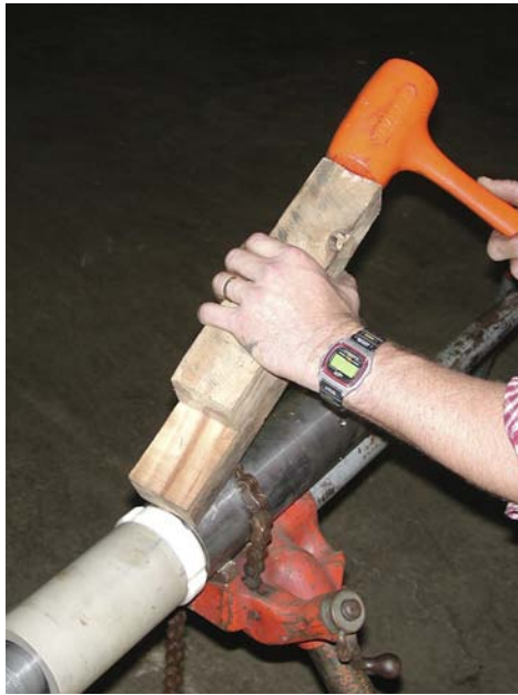
Figure 14. How to remove the antenna coil assembly.
