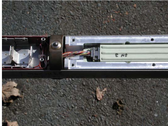
Figure 13. With the cover plate removed, the encapsulated PC board is revealed.
