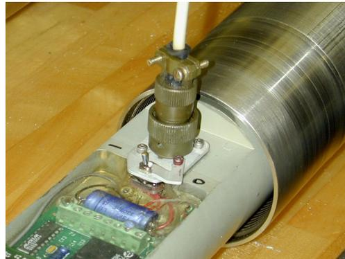
Figure 6. Close-up of the modified RS-232 serial cable connected to the DSA-XM’s electronics module. Note also the power switch in front of the connector.
