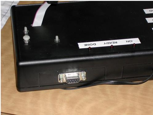
Figure 5. Serial port of the DSA-XM Memory Reader. The serial port shown here should be connected to the 2-port serial data switch.
