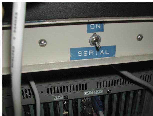
Figure 8. The serial switch on the back of the PC DAS.
