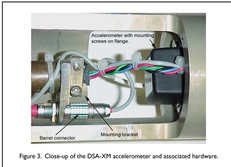
Figure 3. Close-up of the DSA-XM accelerometer and associated hardware.
