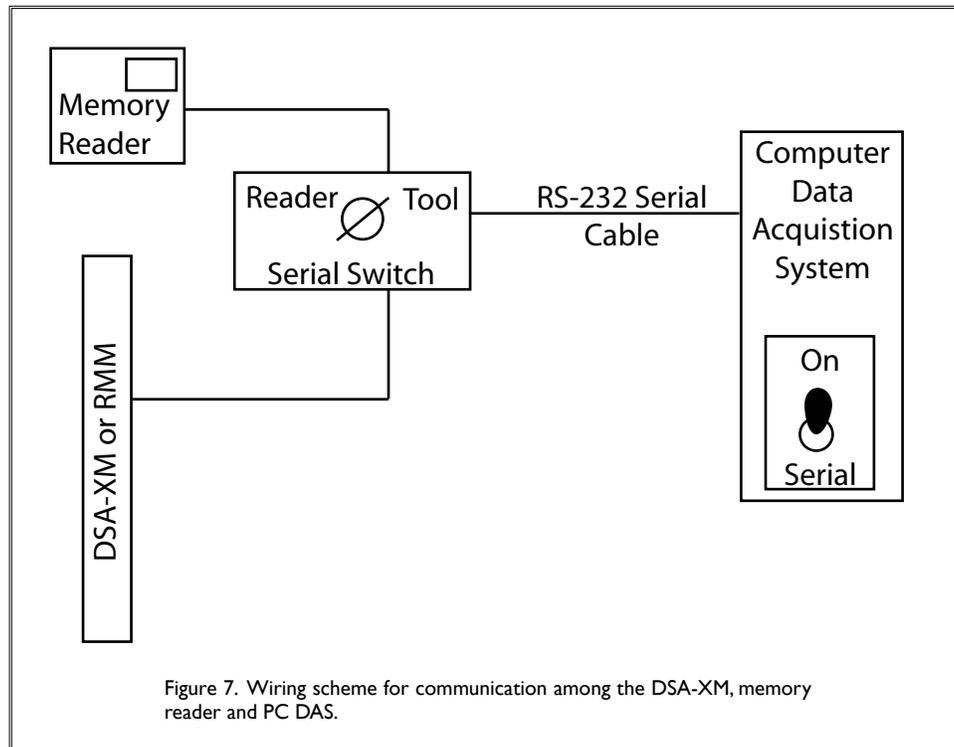
Figure 7. Wiring scheme for communication among the DSA-XM, memory reader and PC DAS.
