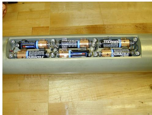
Figure 2. Battery compartment with 6 AA batteries.
