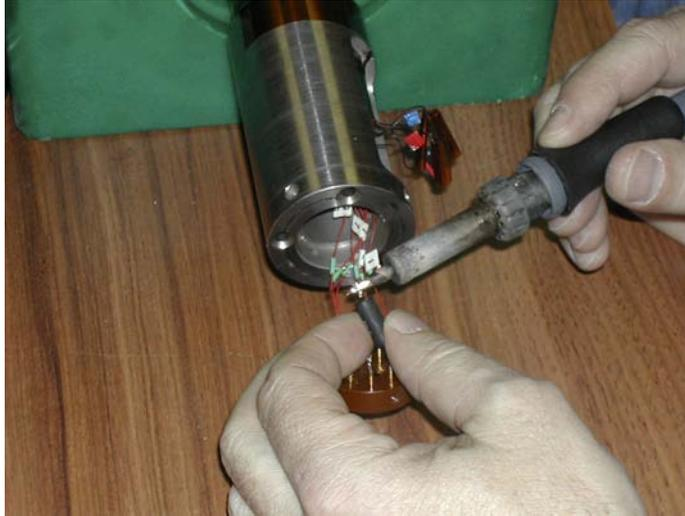
C. Remove the tape that is on the conductors and unsolder the wires:
