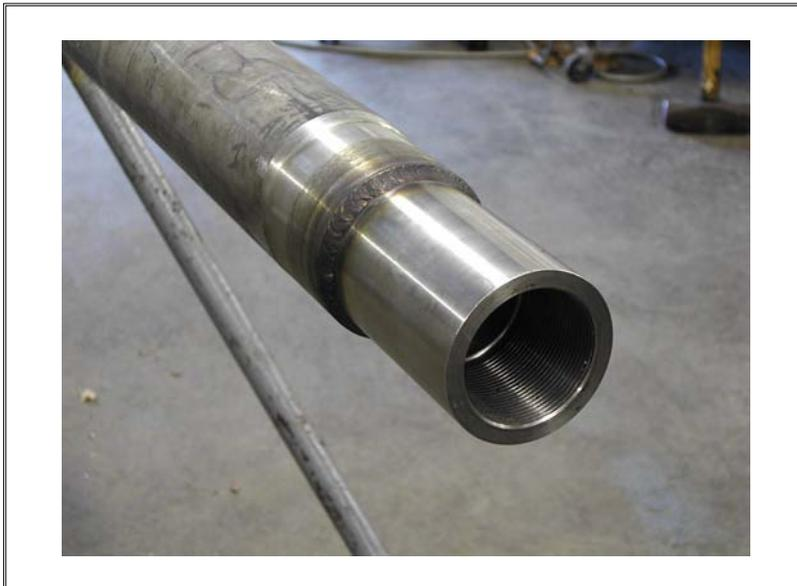
Below is a picture of the lower housing with the lower chassis attached. To remove the lower chassis, use a pin spanner wrench to loosen the threaded collar at the lower end of the HTT housing. The collar is located between the housing and lower end cap, which are both indicated with red alignment grooves.
