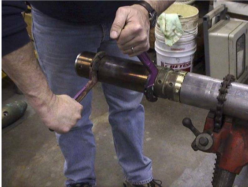
Figure 6. Tightening the top connector.
