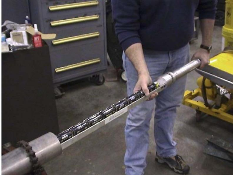
Figure 4. Sliding the battery cartridge back into the tool.
