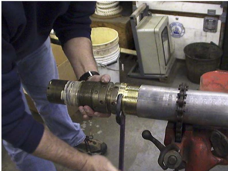
Figure 3. Unscrewing the assembly from the tool.
