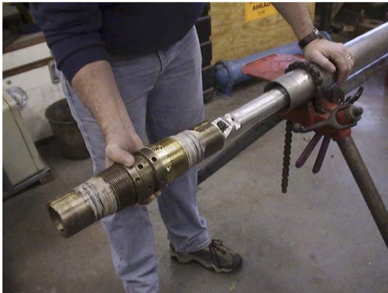
Figure 5. Aligning the cartridge's pinholes with the tool chassis's pins.
