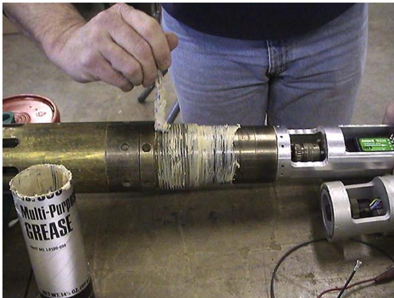
Figure 2. Application of Lubriplate 930 grease after replacement of the O-rings.
