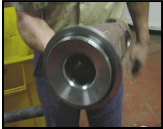
Now, pull out the solenoid valve block. The instructions for servicing the solenoid are on the PORT wall in the lab. Be gentle with it when pulling it out –do not go and scratch it with a wrench if it is stuck!
