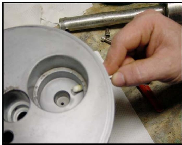
Clean the distributor with care, there are two O-rings **143** & **139** on the outside that you have to service, too. Remember to grease the holes on the end before you re-assemble the distributor.
