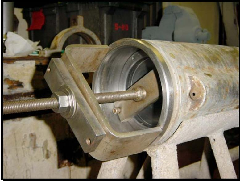
Now you have all the parts out of the gun body. It is time to start servicing them. We will take the sleeve **102** first. Place it on a piece of paper towel. Clean it well. Use oil or grease if needed, and a green scrub pad. Make sure not to scratch it.
