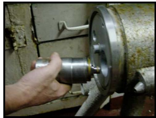
There should always be serviced solenoids in the top drawer of the underway lab work bench. The clean ones will be in zip-lock bags with the Leg number. The two O-rings that go on the outside of the solenoid will be in the bag, so all the parts that go on this solenoid will have been checked out. All you need to do is to apply some Dow Corning 111 Compound on the outside of the solenoid, grease the two O-rings in the bag and put them in place.
