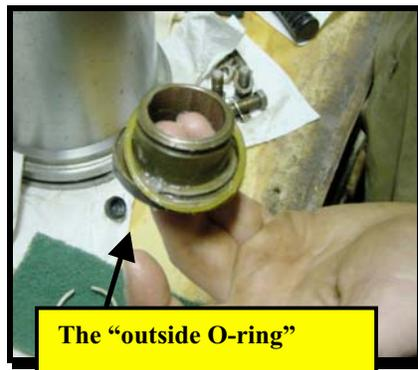
Clean and grease the base, and put everything back together. Remember to bend the “wings” on the lock washers back up.
