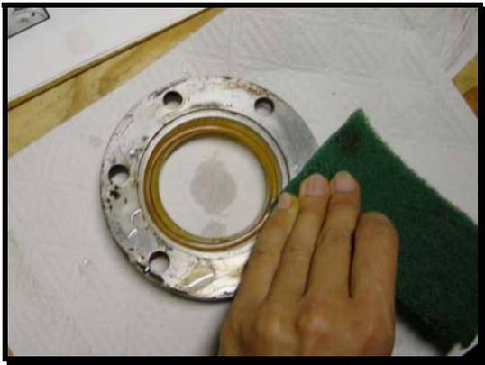
Clean the connecting surfaces between the clamp and the sleeve body well. Remove the yellow sealing ring **104**.
