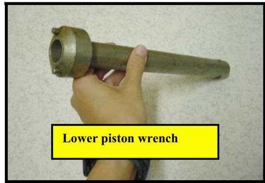
Find crank handles for the piston wrenches. The hex wrenches in the S-80 tool box work well for this. On the next page, a drawing shows which wrench is for which end.
