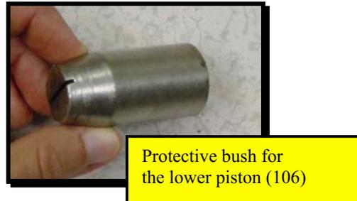
Screw the protective bush (picture) on the lower piston. Now you can carefully tap the piston 106 with the handle of the rubber mallet, if it does not want to come out by just pushing with your hand. **DO NOT LET IT FALL OUT!** If you have someone with you, ask this person to stand at the other end of the gun in order to hold on to the piston when it starts coming out.
