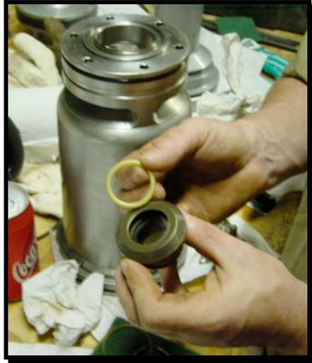
Clean the bearing and grease it. Q-tips are very useful for cleaning the O-ring grooves. Clean and grease both the O-ring and the black split ring on the inside of the bearing. Put them back in place. Next, service the “outside O-ring” **136** and then re-assemble it.
