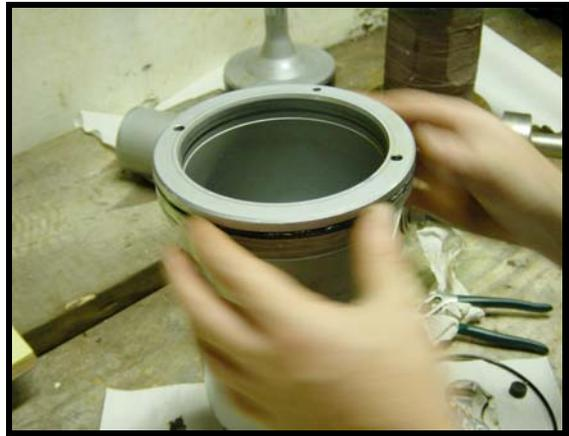
Clean the O-rings. If they are damaged, replace them with new ones. Clean grooves. Grease the grooves with Dow Corning 111 Compound and then, grease the O-rings and put them back in place.
