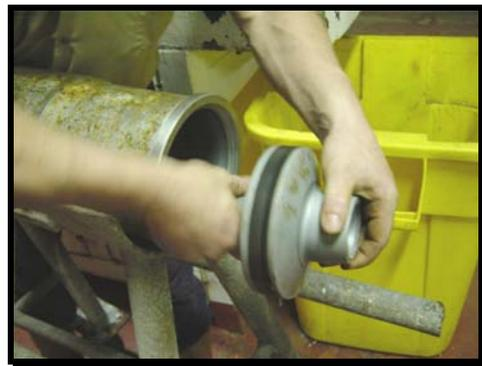
Next, pull out the sleeve. The same tool is used for this as was used for pulling out the distributor. Same story, be careful with it and hold on to the threaded part of the extractor so the sleeve does not fall and hit itself.
