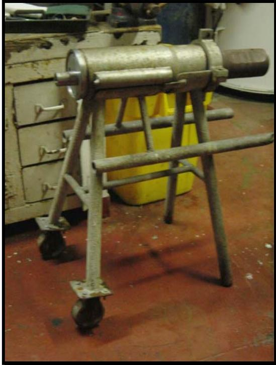
Push the cart over to the workbench. Again, have someone hold the damper while you detach it by removing the clamp. The damper is **HEAVY** too.
