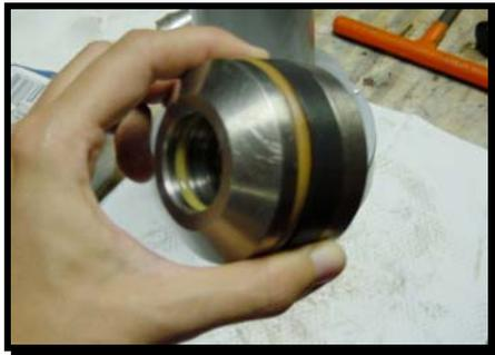
On the upper piston, there are an O-ring **142** and a split ring **132** on the outside, and an O-ring **140** on the inside. Clean all these and check their condition. Replace if needed, grease the piston and the O-rings. **Remember to clean the piston wrenches** before screwing the piston back in place, so you do not put any gunk from the dirty gun into the clean one.
