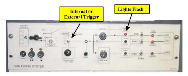
Now you are ready to send the trigger signal to the gun. Select which gun you want to test, PORT/STBD/AUX or a combination and turn ON the appropriate switches. The lights for whichever triggers you have selected should flash.
