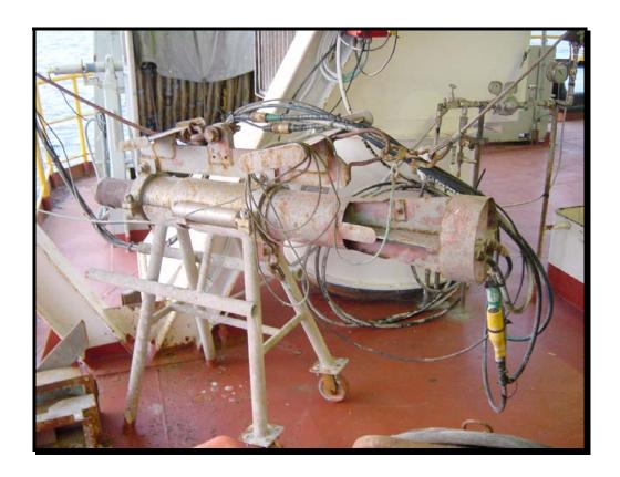
Go to the fantail. Make sure the pressure gauges are all showing zero and that the valve handle is perpendicular to the air line (the air is OFF). Connect the gun solenoid to the trigger lead on the red box (the trigger needs a closed circuit to fire).
