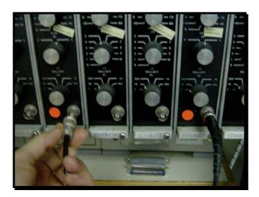
3) Set the amplifiers on 30, Gain on 5 and Low Freq Rolloff to 1 Hz.
