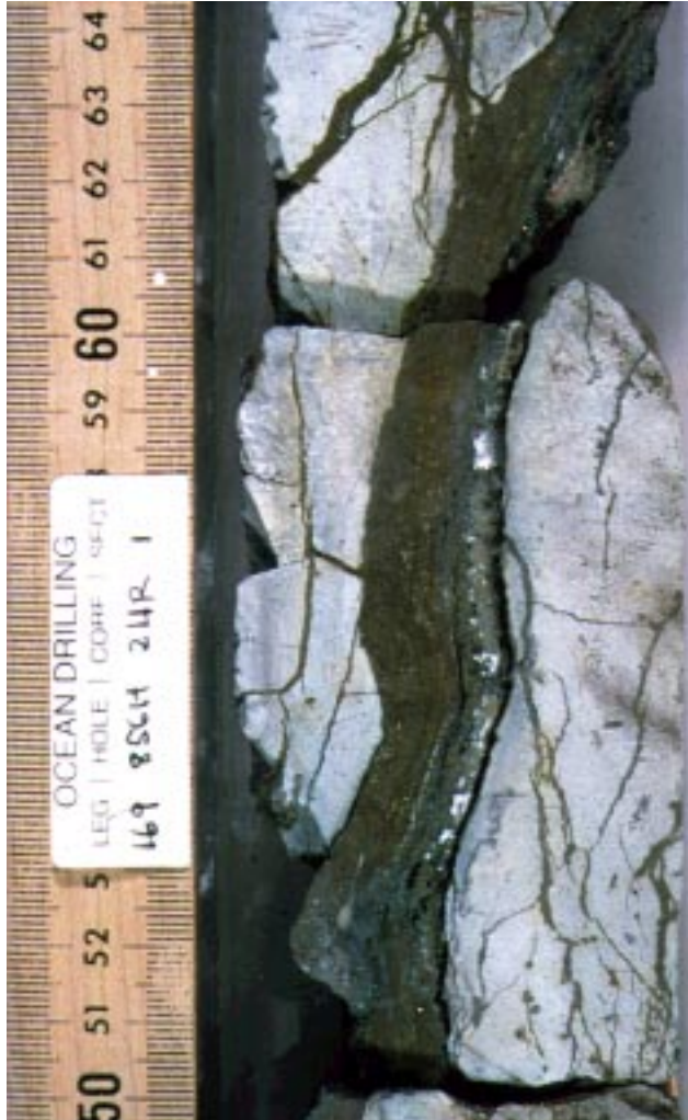
Figure 2. Pyrrhotite-isocubanite-chalcopyrite veins cutting lithified mudstone in the Cu-rich feeder-zone mineralization that immediately underlies the Bent Hill massive sulfide.
